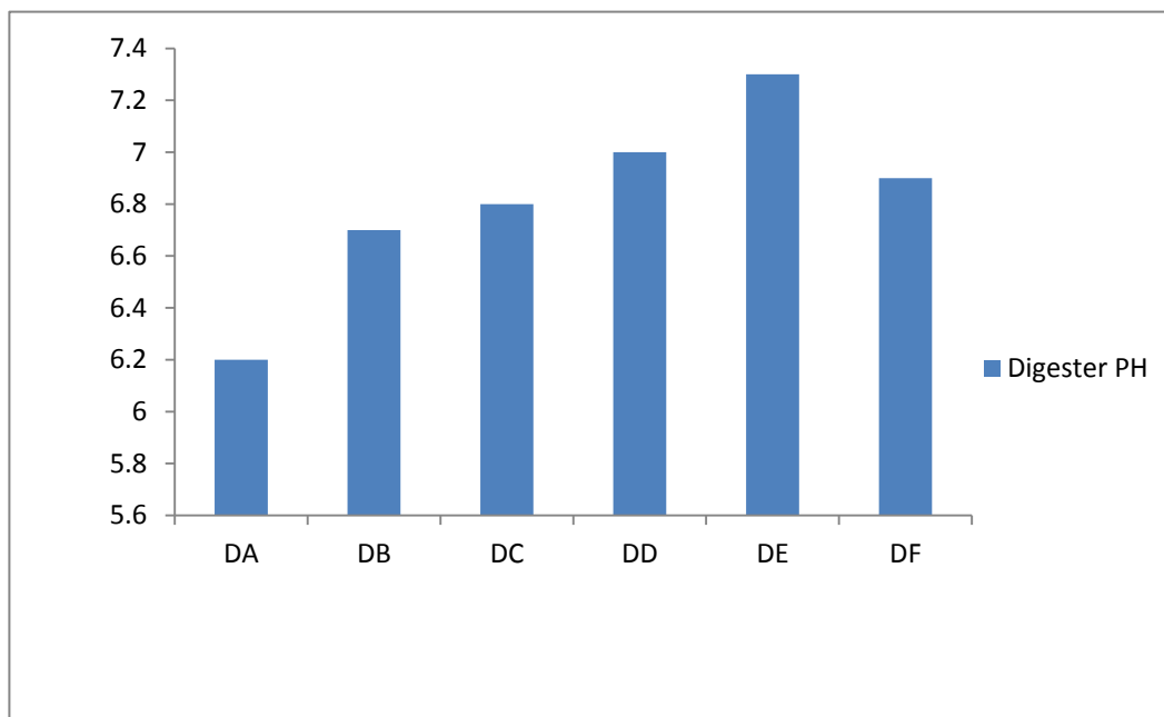
Figure 1: The pH of substrate in each of the digesters before digestion.
