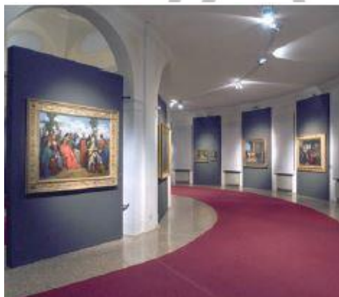
Fig. 8.0: The directional light of spot lamps raises the brightness for exhibits – here with an appropriate beam angle for paintings.
