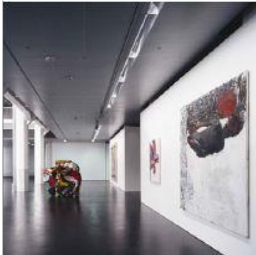
Fig. 7.0: Wallwashers distribute their light asymmetrically.
