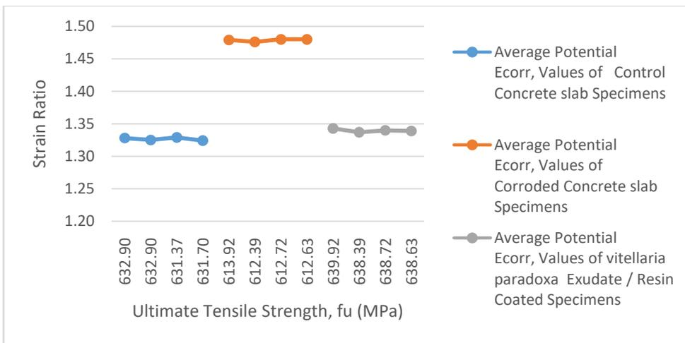
Figure 3.3A: Average Ultimate Tensile Strength versus Strain Ratio
