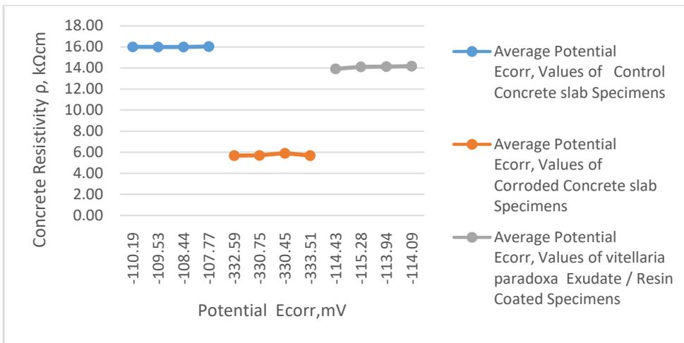
Figure 3.1 : Average Potential E<sub>corr</sub>, Values of Control Concrete slab Specimens, Corroded Concrete slab Specimens, and Vitellaria paradoxa Exudate / Resin Coated Specimens
