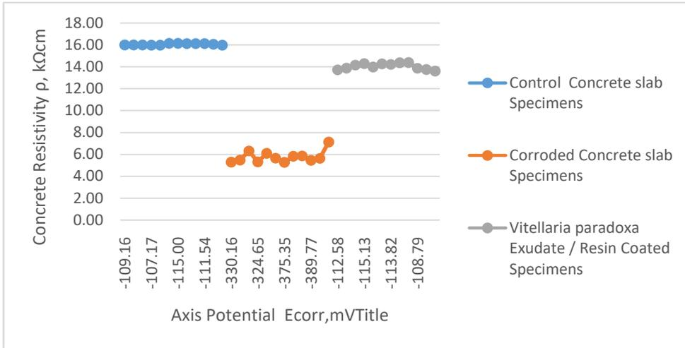
Figure 3.1 : Concrete Resistivity ρ, kΩcm versus Potential E<sub>corr</sub>,mV Relationship
