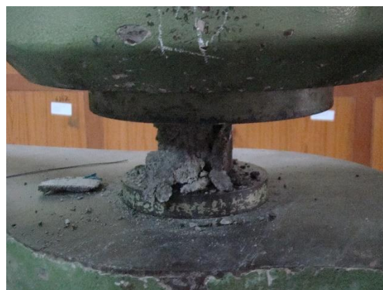
Fig 6. Cube after failure
