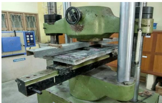
Fig 8. Ferrocement Panel setup
