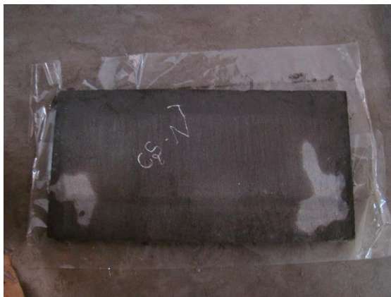
Fig 7. Demoulded Ferrocement panel
