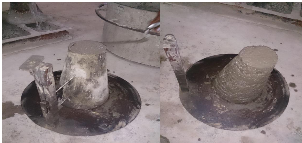
Figure 2.3. Fresh concrete filled in the mould and after removal of mould
