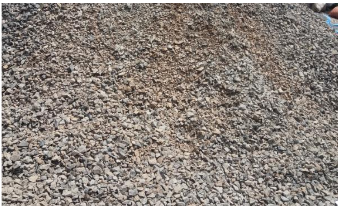
Figure 3.4. Coarse Aggregate with high Flakiness, high aggregate crushed value, and clay particles
