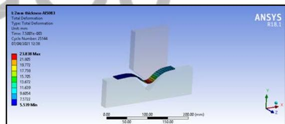
Figure 22: deformation at 0.75 ms
