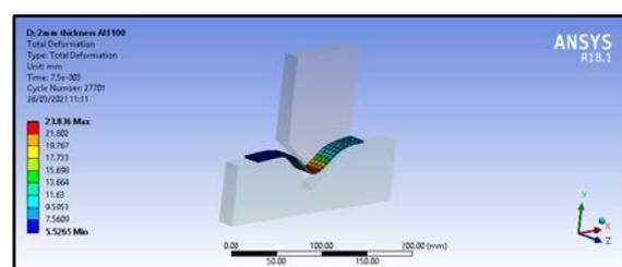
Figure 12: deformation at 0.75 ms
