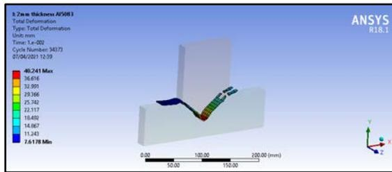
Figure 24: deformation at 10 ms.
