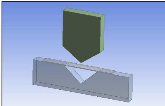
**Figure 2:** CAD modeling of die, punch and sheet metal using ANSYS design modeler.
