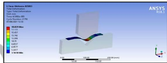
Figure 21: deformation at 0.65 ms
