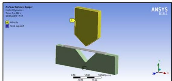
**Figure 5:** Loads and Boundary Conditions.
