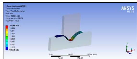
Figure 23: deformation at 0.9 ms.
