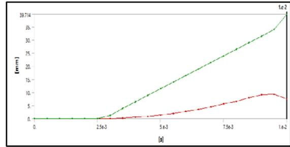
Figure 15: deformation vs time curve for Al-1100 material.
