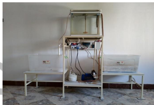
Figure 2. Sequencing Batch Reactor System (SBR)
