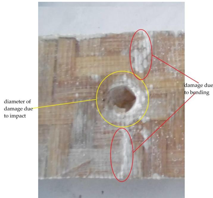
Figure 3 Impact damage and post-impact bending
