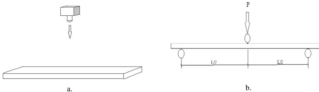
Figure 2 Schematic a. dropweight impact b. three point bending test.
