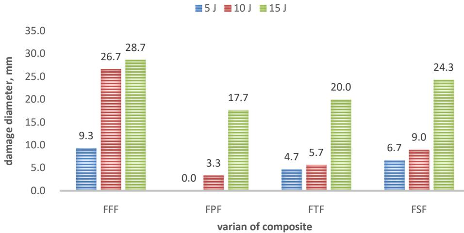
Figure 4 Diameter of impact damage on composites
