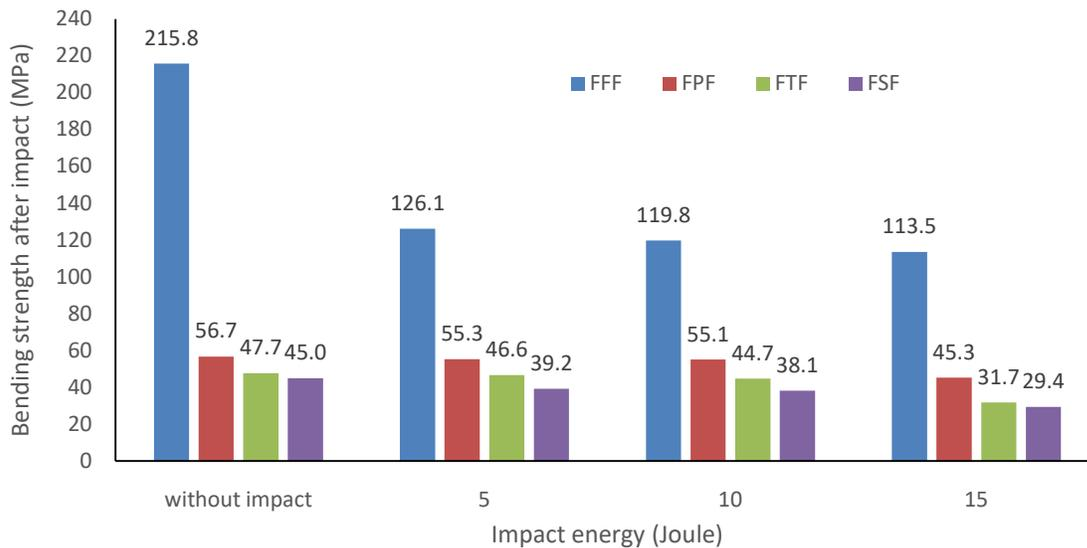
Figure 5 Composite bending strength after impact
