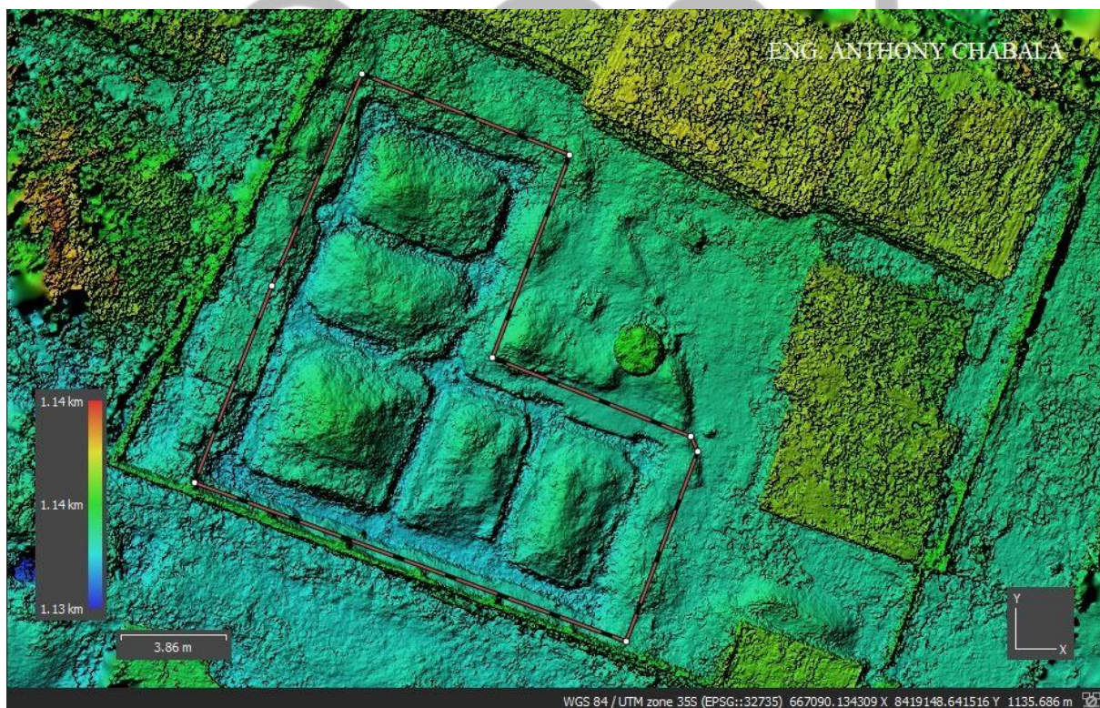
Figure 6: A DEM for X, Y and Z coordinates of the project area as bound by the line. Footing put up with soil materials remaining only on the spaces where rooms are to be built.
