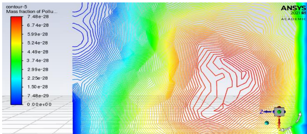
Figure 16. Contours plot of NO x Mass Fraction—Prompt and Thermal NO x Formation of dual GDI
