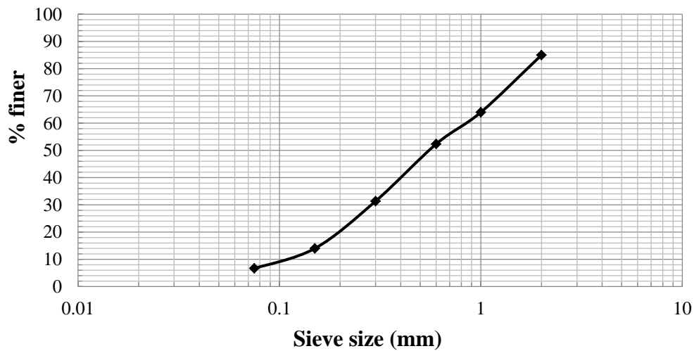
Figure 3.1 Particle Size distribution curve of BCS
