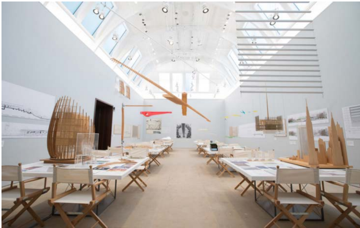
Figure 2.16 efficient use of double clerestory toplight as daylighting strategy in exhibition space. (Arup, 2021)
