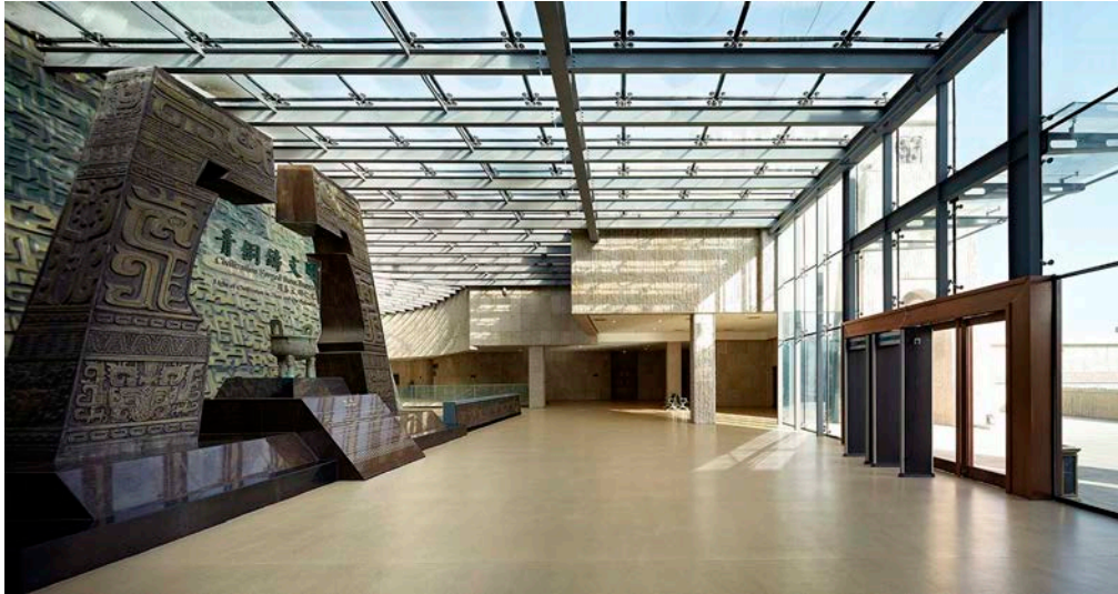
Figure 2.11 Combination of full glazed flat-roof skylight and glass Walls for natural/daylighting. . Image Source: (Chen) as cited in (Shuang, 2020).
