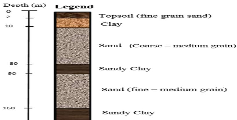
Fig. 20 Typical borehole log of Katuzo in Gashua (Modified from Ministry of Water resources Damaturu).
