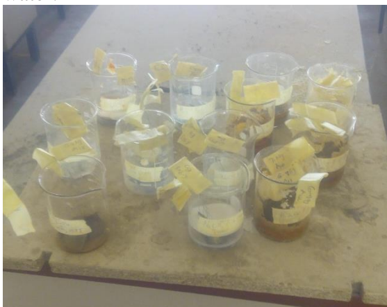
Figure 2: Submerged mild steel samples ready for taking of readings
