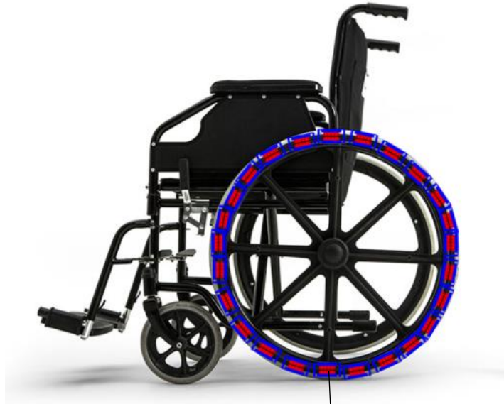
Figure 1: Piezoelectric crystals implented within the inner surfaces of the tires on a wheelchair
