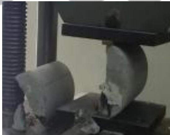
Figure 3: Splitting tensile test
