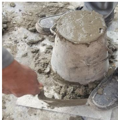
Figure 1: Slump Test for fresh concrete
