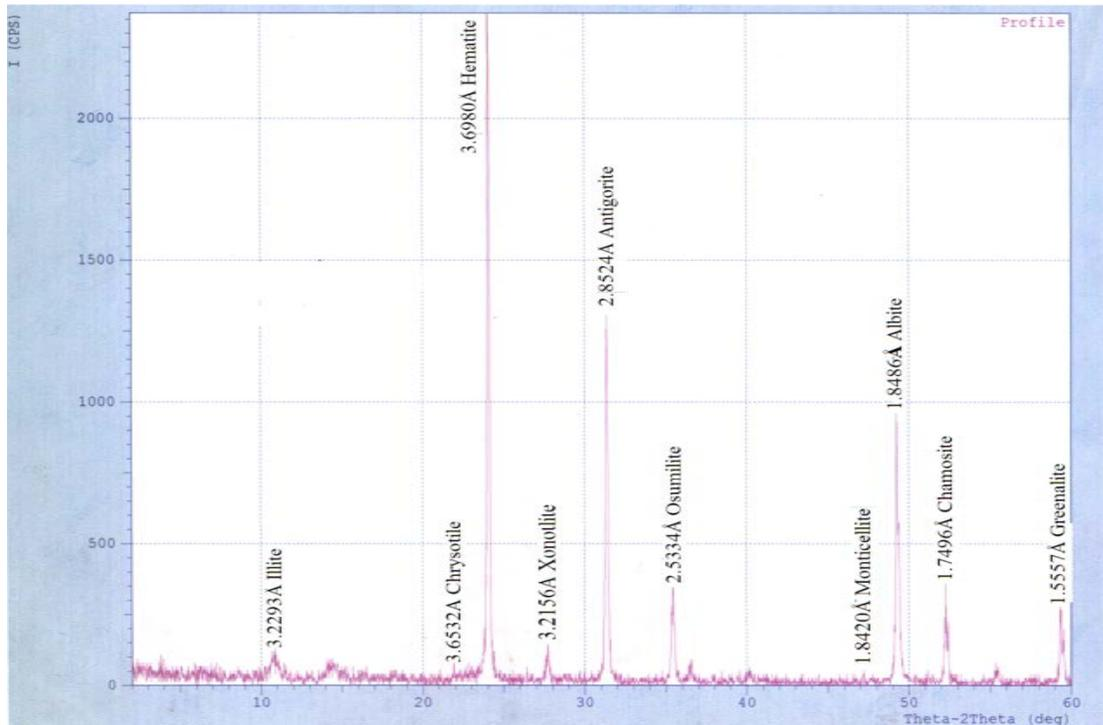
**Fig. 1.2: X-ray diffractograms of clay sized particle of soil F1**
