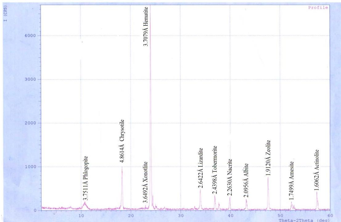
**Fig. 1.3: X-ray diffractograms of clay sized particle of soil F2**
