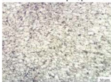
Fig. 3.9: Control sample (Pure Aluminium)
