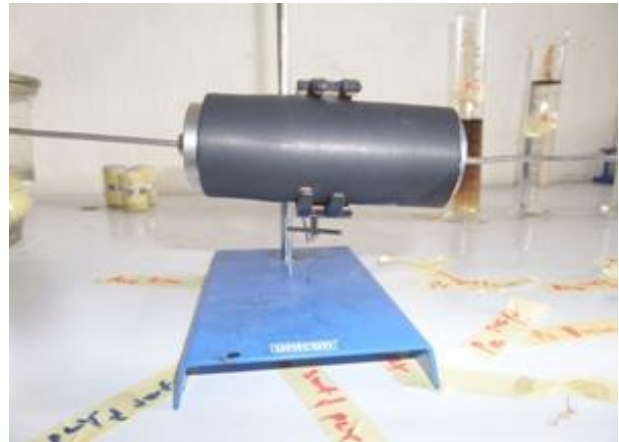
Figure 3.7: Sand Holder fitted with end-stem
