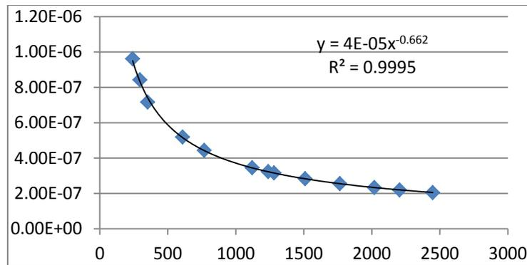
Figure.2 The absolute energy peak efficiency measurement using the standard sources <sup>226</sup>Ra and <sup>60</sup>Co
