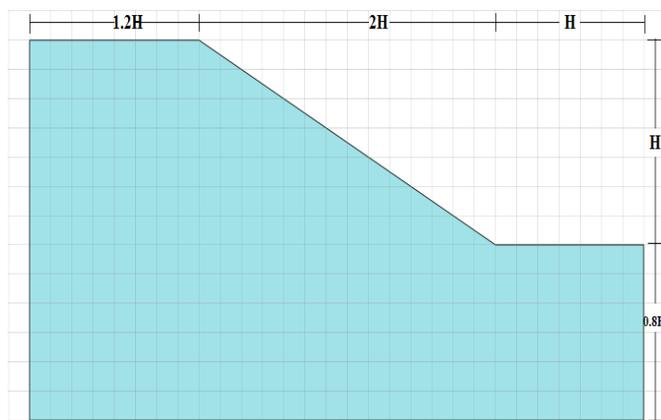
Figure 2: Plaxis 2D model and Geometry, H=7m.
