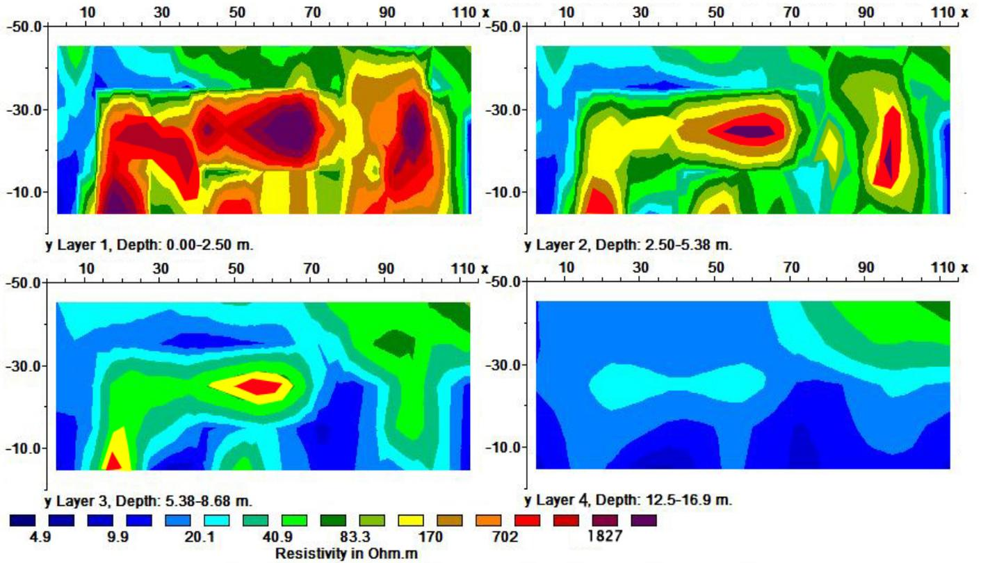
Figure 9 and 10 display results from the control unit taken 2.17kilometers away from the oil spill source. The result shows no contamination.
