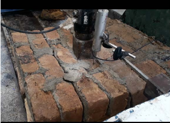
Figure 7 cracked specimen of masonry panel.
