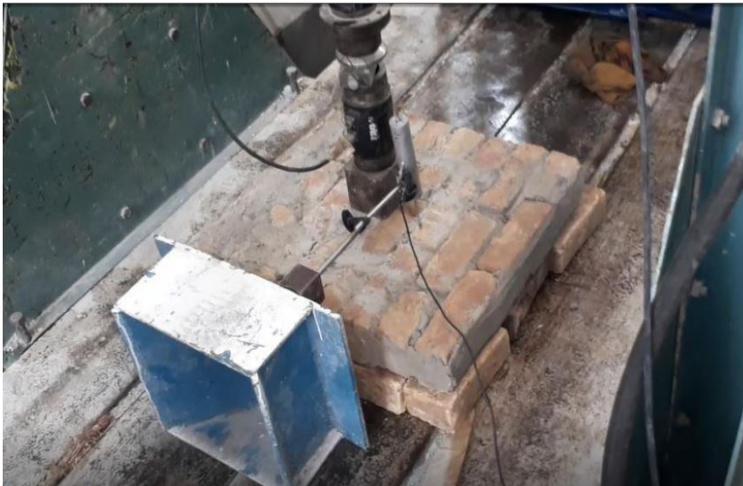
Figure 5 Test setup for out-of-plane shear
