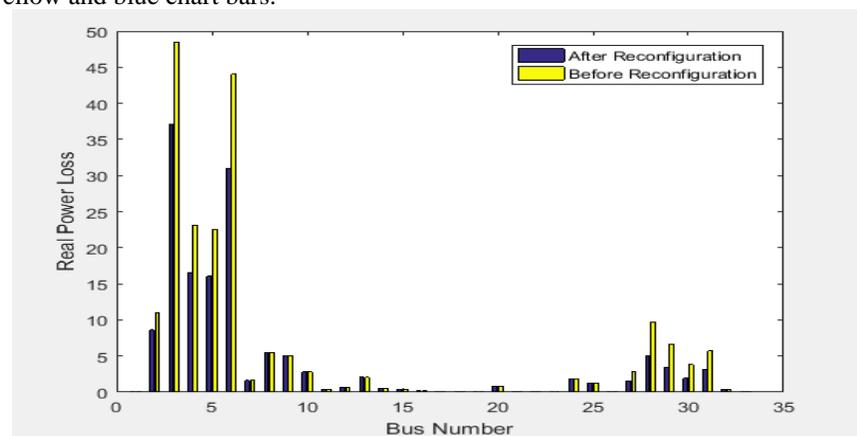
Figure 7: Real Power Loss for 33-Bus IEEE Radial Distribution Network before and after Reconfiguration using Firefly Algorithm.
