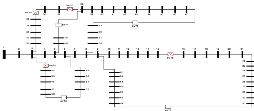
Figure 9: Doma 69-Bus Distribution Network before Reconfiguration.
