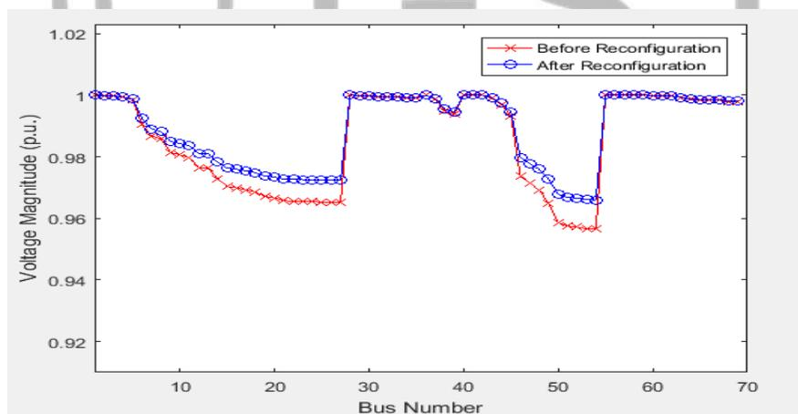
Figure 13: Voltage Profile Improvement for DOMA -69 Bus Radial Distribution Network after Reconfiguration using Firefly Algorithm
