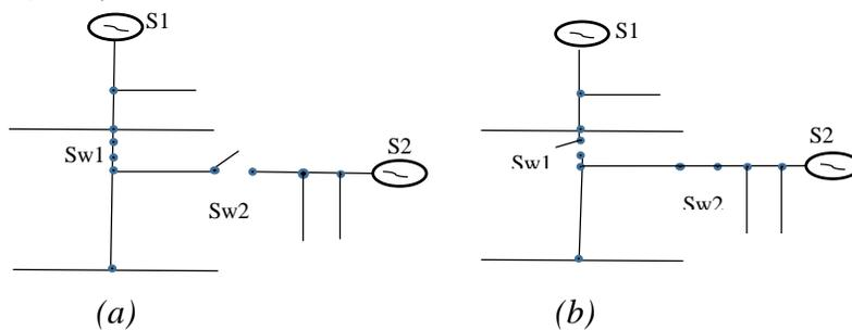
Figure 1: simple illustration of a network reconfiguration. (Dias *et al.*, 2022)
