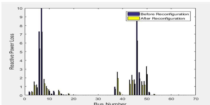
Figure 12: Reactive Power Loss for DOMA -69 Bus Radial Distribution Network after Reconfiguration using Firefly Algorithm.
