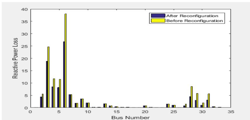
Figure 6: Reactive Power Loss for 33-Bus IEEE Radial Distribution Network before and after Reconfiguration using Firefly Algorithm
