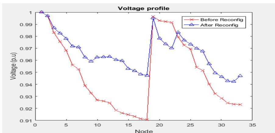
Figure 8: Voltage Profile Improvement for 33-Bus IEEE Radial Distribution Network after Reconfiguration using Firefly Algorithm
