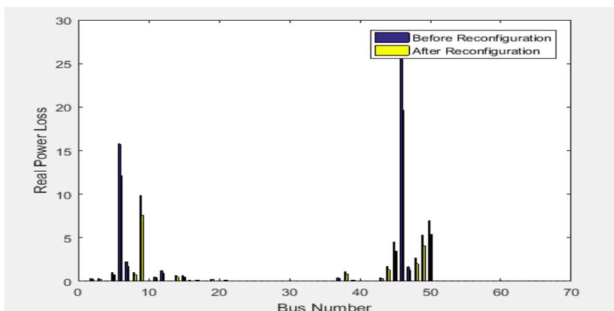
Figure 11: Real Power Loss for *DOMA -69 Bus Radial Distribution Network* after Reconfiguration using Firefly Algorithm
