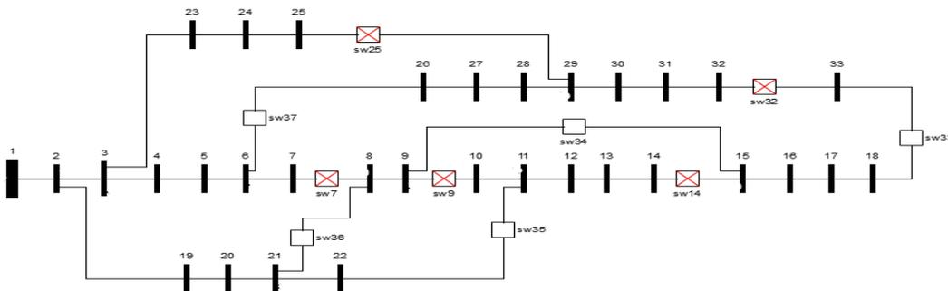
Figure 4: IEEE 33-Bus Distribution Network before Reconfiguration
