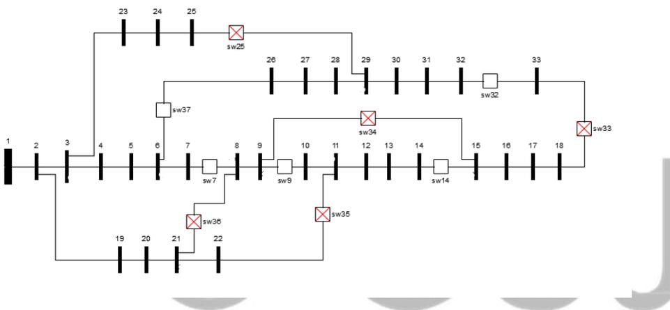
Figure 5: IEEE 33-Bus Distribution Network after Reconfiguration
