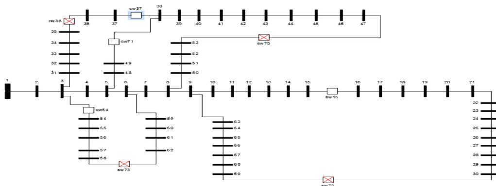
Figure 10: Doma 69-Bus Distribution Network after Reconfiguration
