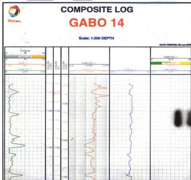
Figure 3. A typical wireline log of GABO well 14
