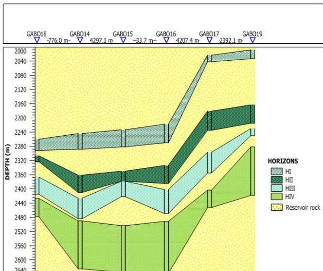
**Figure 10. Fence-diagram showing the four horizons**
