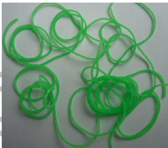
Figure 3. Uniformity of the extruded composite filaments. Source: The authors
