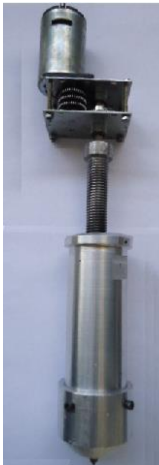
Figure 6. Constructed complete extruder device. Source: The authors
