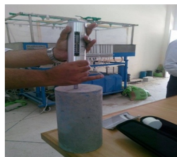
Figure 5: Schmidt hammer test
