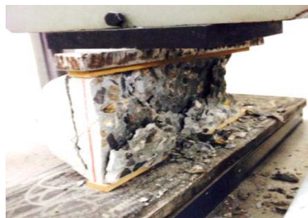
Figure 3: Split tensile test (after splitting)
