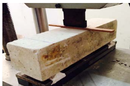
Figure 4: Flexural test (three point loading test)
