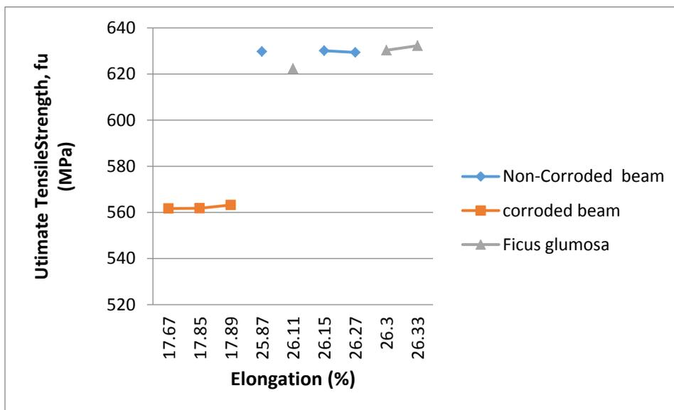
Figure 3.3: Average Ultimate Tensile Strength versus Strain Ratio of Beam Specimens (Non-Corroded, Corrode and Resin Coated Specimens)
