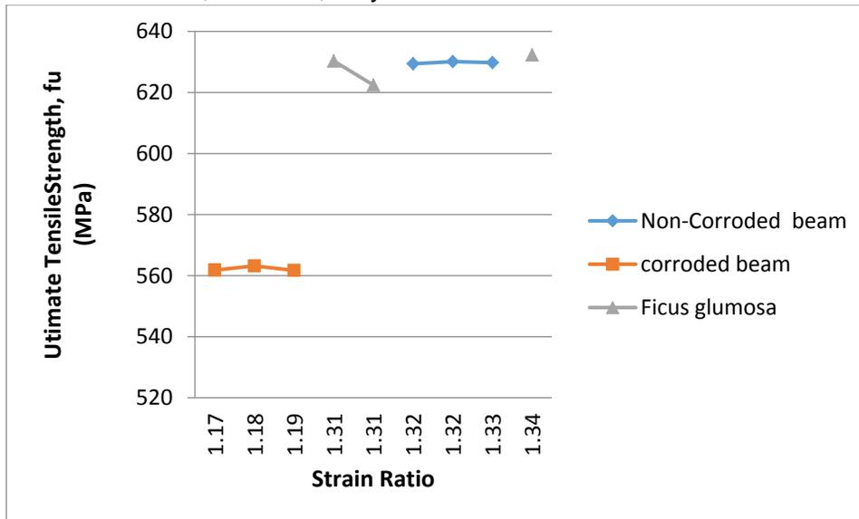
Figure 3.5: Average Ultimate Tensile Strength versus Elongation of Beam Specimens (Non-Corroded, Corrode and Resin Coated Specimens)
