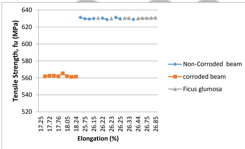
Figure 3.2: Ultimate Tensile Strength versus Elongation of Beam Specimens (Non-Corroded, Corrode and Resin Coated Specimens)
