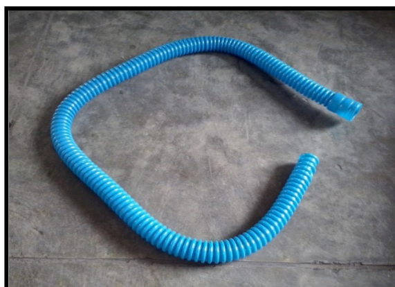
Tube used to connect the water pump and the tracks
