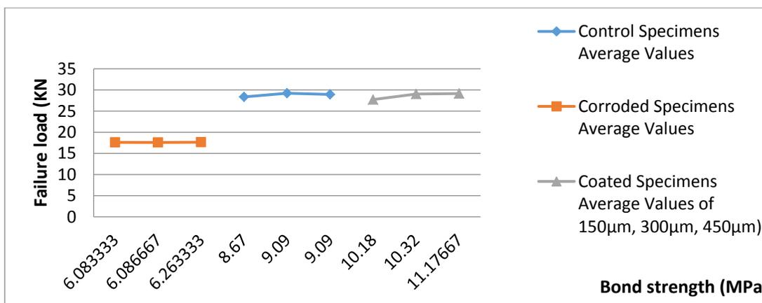
**Figure 3.2: Average Results of Pull-out Bond Strength Test ( $\tau$ ) (MPa)
