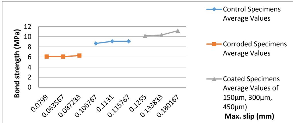
**Figure 3.4: Average Results of Pull-out Bond Strength Test ( $\tau$ ) (MPa)
