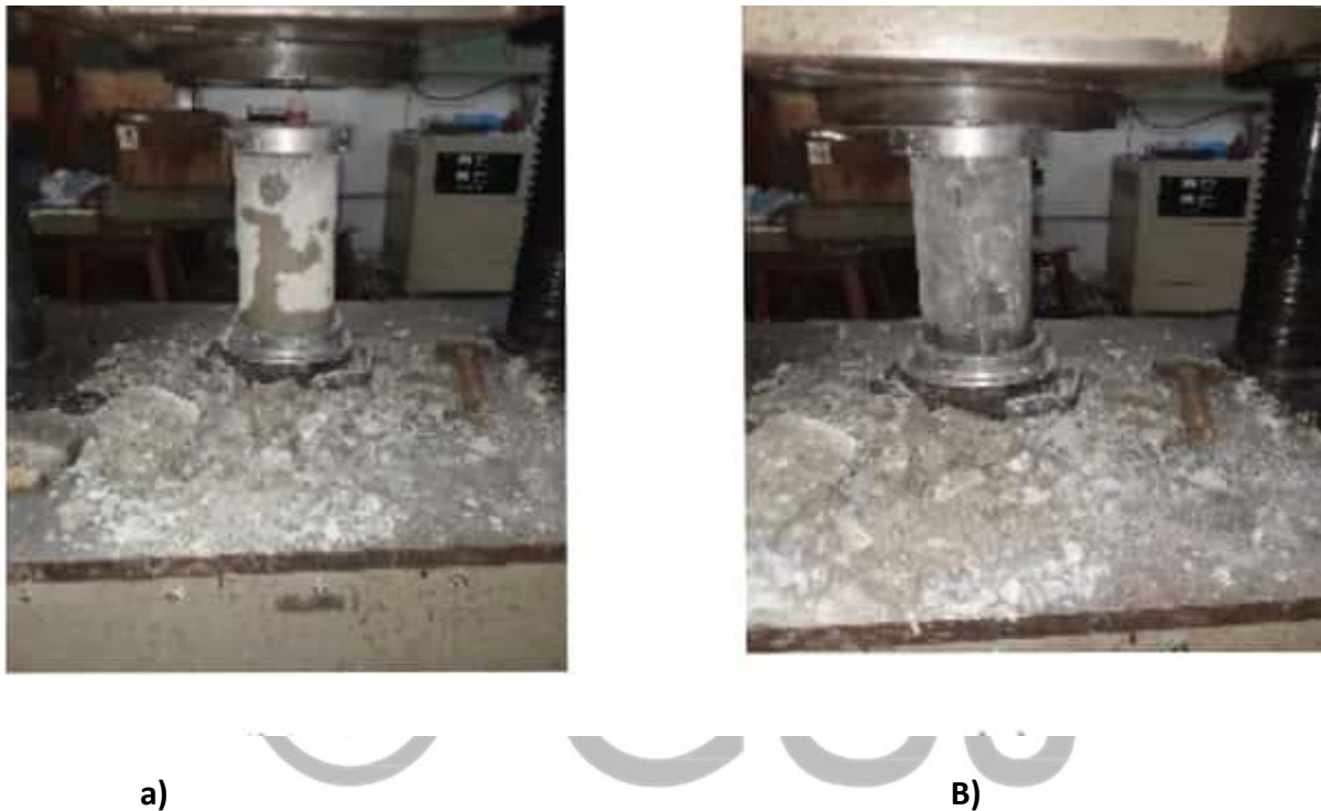
Figure 3.6.a,b,concrete compressive test in UTM
