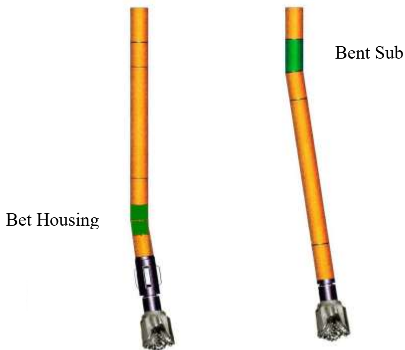
Figure 2.7: Positive Displacement Motor with Bent Sub and Bent Housing [4]
