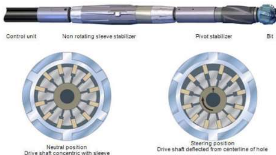
Figure 2.8: Modes of Rotary Steerable System
