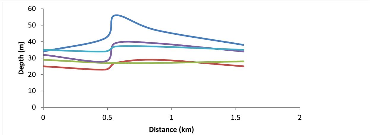
Figure 2a: Combined Flow Depth Hydrographs for River Valley
