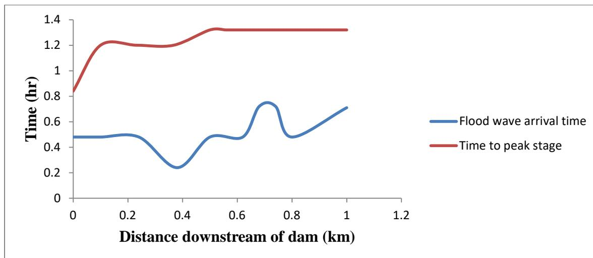
Figure 3b: Time of wave to peak stage
