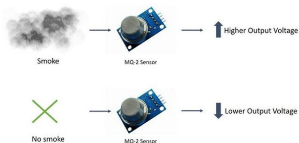
Fig21. Working principle of gas sensor
