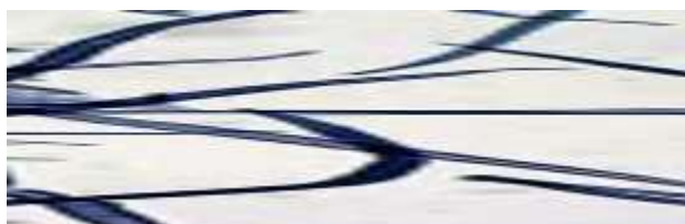
Figure 2. Bamboo fiber obtained on a visopam microscope
