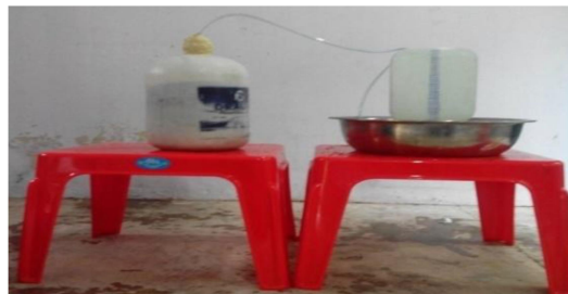
Fig 1 Preparation of effective microorganism solution and production of biogas
