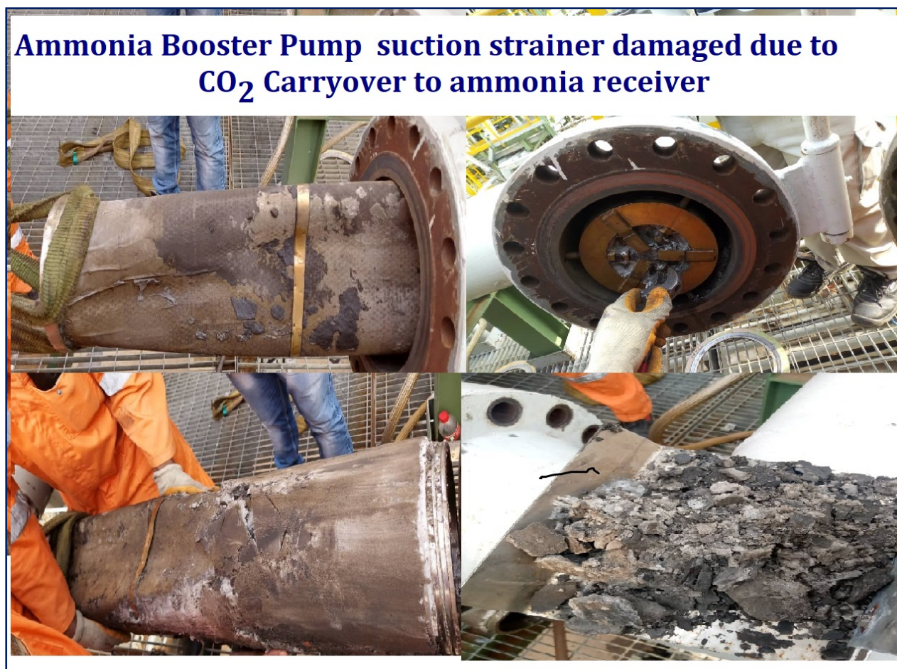
Fig-12(ammonia booster pump strainer damaged)
