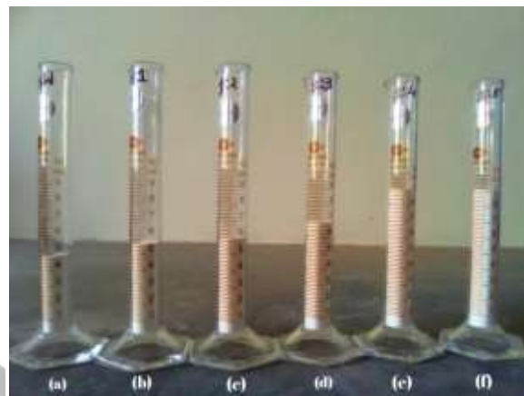
Figure 8: Volume occupied upon tapping by 3YSZ powders calcined at 100°C wherein the precipitate were washed with water and different amounts of propanol; Water-washed powder (a) and propanol-washed powders (b) 1:1 (c) 1:2 (d) 1:3 (e) 1:4 & (f) 1:5 water to propanol amount ratio.
