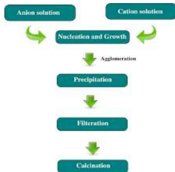
Figure 2:Flow chart of Co-precipitation method
