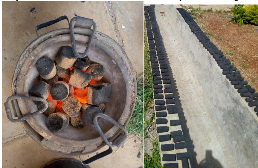
Charcoal briquettes made from charcoal dust and waste paper or cow dung
