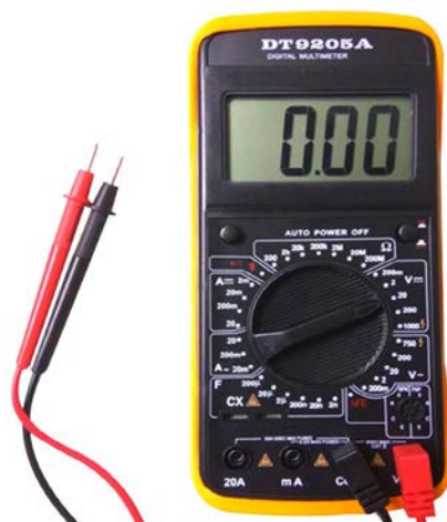
Figure 4: Employed digital multimeter
