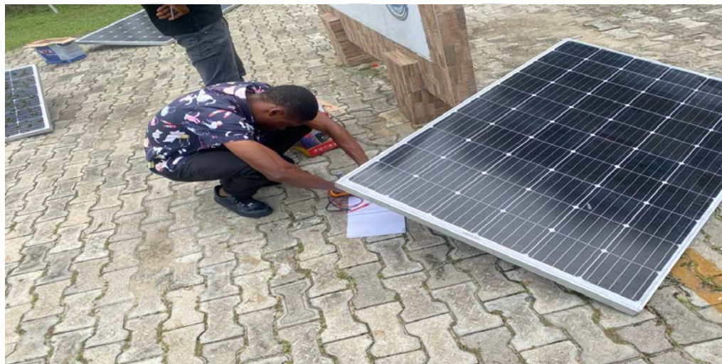
Figure 3: Experimental setup for solar panel without soot (control).
