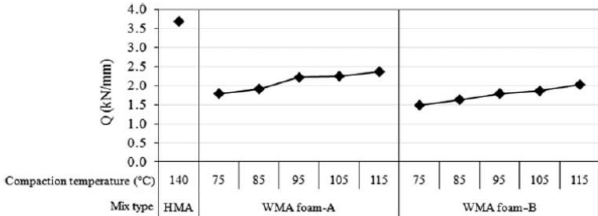
Fig.2 WMA foam mixes with control HMA -Q values comparison
