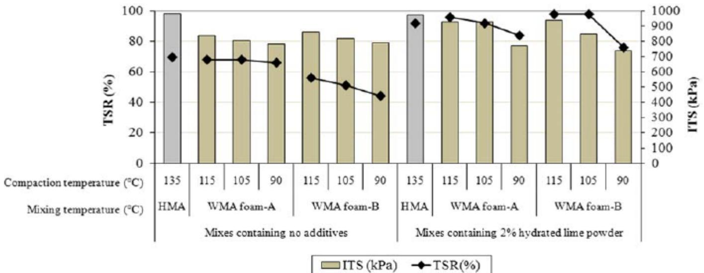
Figure 1. Comparison of dry ITS and TSR values of WMA foam mixes with control HMA
