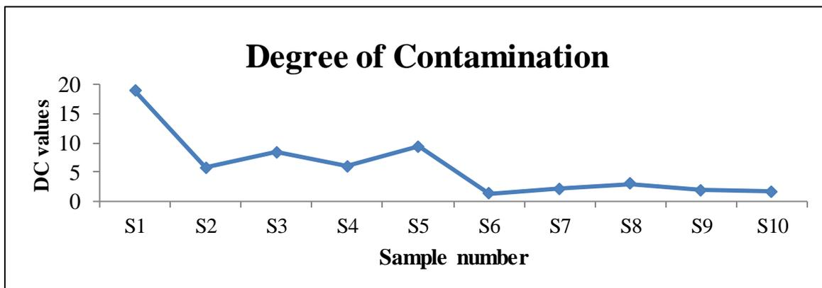
Figure 7: The degree of contamination of trace elements in the water samples in Nkongsamba
