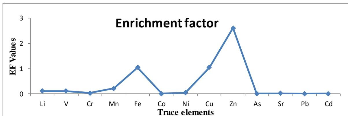
Figure 8: The enrichment factor for trace elements in the water samples in Nkongsamba
