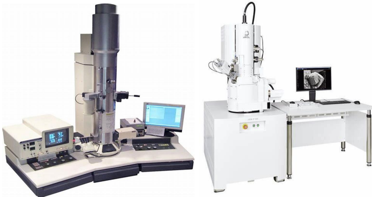
(a) Transmission Electron Microscopy (TEM) (b) Scanning Electron Microscopy (SEM)
