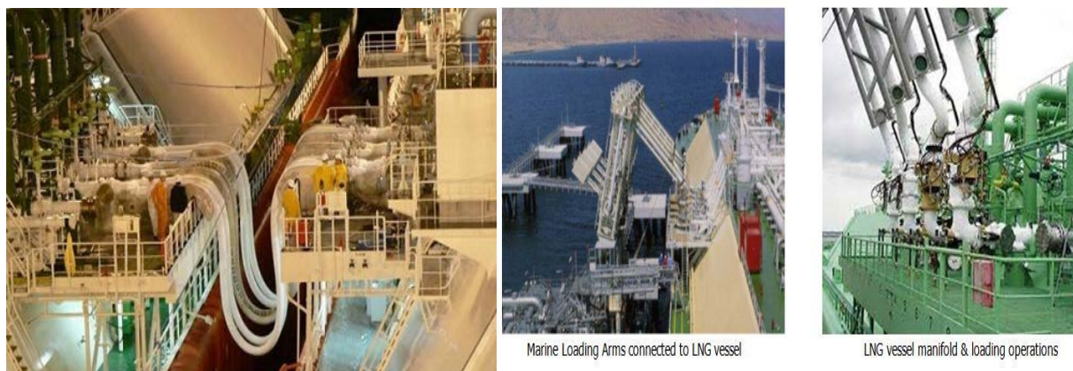
Fig 7: Two images of loading gas cargo of atypical LNG Carrier 47,48
