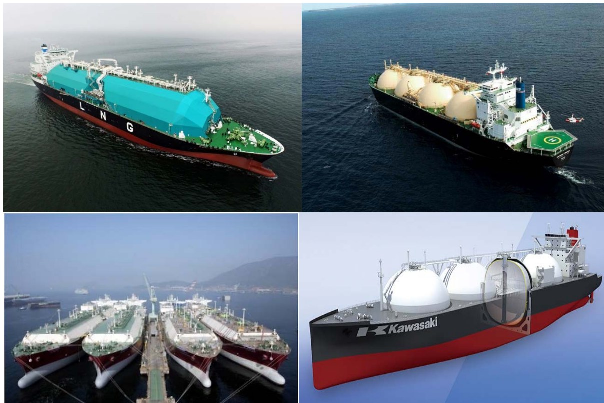
Fig 8: Example of few tank and dome type LNG Carrier 52,53,54,55
