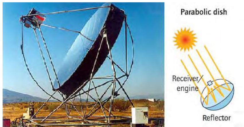
Figure 5-2: Solar parabolic dishes.
