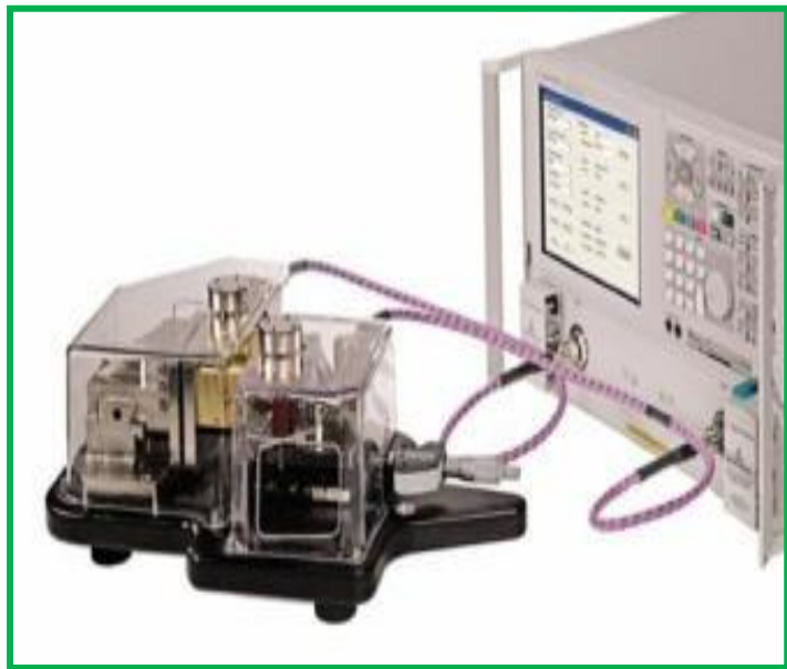
Figure 4.1 Split cylinder cavity resonator setup (Analyser, V.N., 2007)
