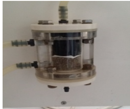
Figure 3.2 Arrangement of the filter media.
