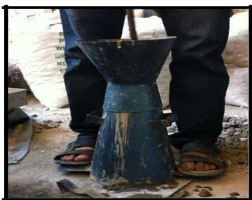
Figure 16: Compacting each layer of fresh concrete
