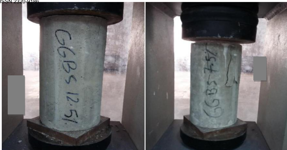
Figure 20: Concrete Cylinder under Testing
