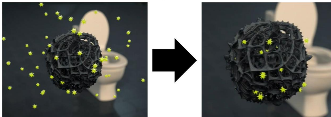
Figure 2: Odor molecules attaching or being adsorbed by the microscopic porous surface area of the Activated Carbon.
