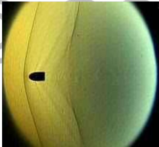
Figure 1.2 Schlieren image of a bullet travelling in free-flight demonstrating the air pressure dynamics surrounding the bullet.
